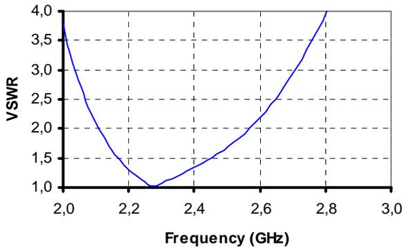
Fig 4 Simulated results of the optimised simple PIFA
