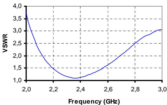
Fig 5 Simulated results of the optimised double PIFA
